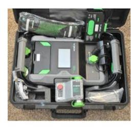
The Used PIM Tester from Kaelus is among the first ever battery-powered PIM Test analyzers in the market. Designed for versatility, this model supports multiple test scenarios – such as testing at the base of the tower, top of the tower, rooftop, as well as in-building for all DAS systems.
